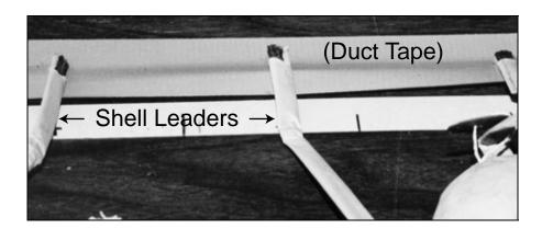
Lay a length of visco fuse or plastic igniter cord on the tape and over the ends of the exposed black match of each shell leader.
