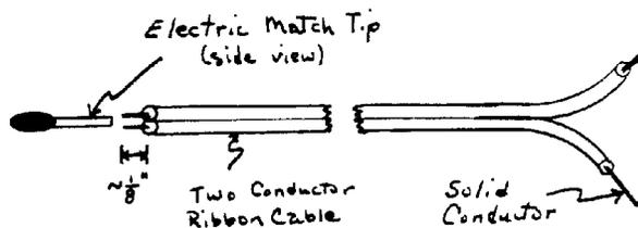
Figure 4. Sketch of two-conductor ribbon cable prepared for soldering to electric match tip.
