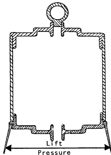
Figure 5. Lift cup expanding.
