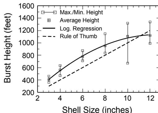
Figure 1. Spherical aerial shell burst height data.
