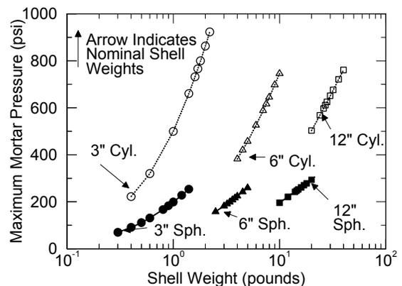
Figure 9. Maximum mortar pressure as a function of shell weight.
