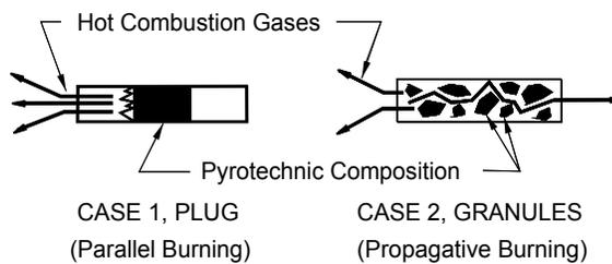
Figure 2. Examples of "parallel" and "propagative" burning.
