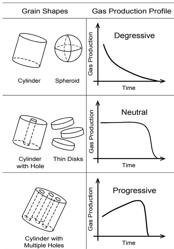
Figure A-1. Propellant powder burning.
