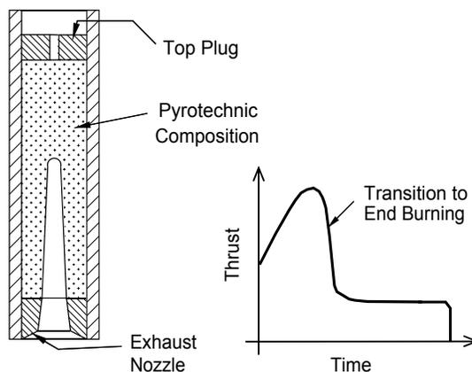
Figure 4. Core burning rocket motor.
