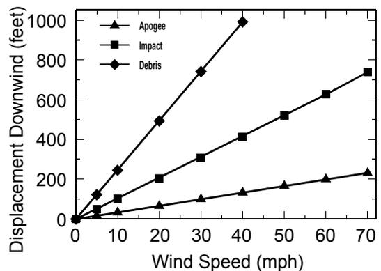
Figure 9. Displacement of 6" spherical aerial shell in wind.
