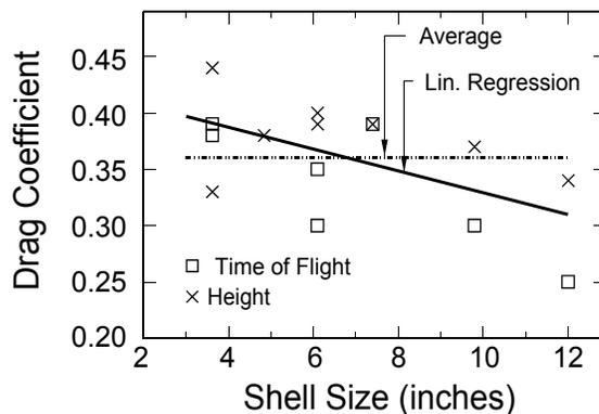
Figure 5. Drag coefficients for spherical aerial shells.
