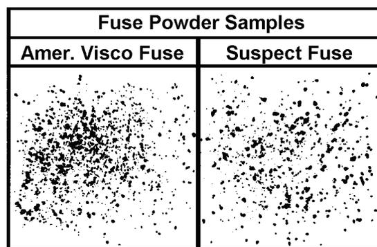
*Photo 1. Photograph of fuse powder extracted from the suspect fuse (right) and normally burning fuse (left).*
