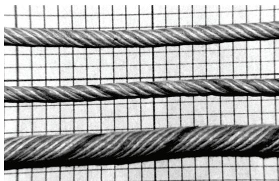
Photo 2. Photograph of three samples of "Instantaneous" fuse shell leaders.
