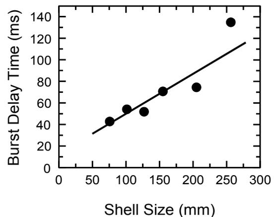
*Figure 7. Average Shell Burst Delay Times as a Function of Shell Size.*
