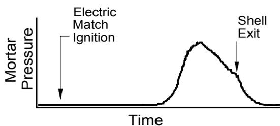
Figure 3. Typical mortar pressure versus time curve for a shell firing.
