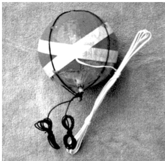
*Figure 5. A typically prepared shell used in measuring burst delay times.*
