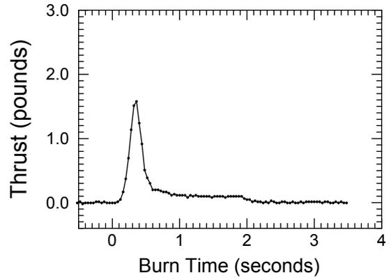
Figure 4. Typical thrust profile of a Sky Bloom rocket.
