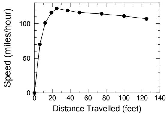
Figure 2. Typical graph of the speed of a Horse Brand sky rocket as a function of distance travelled.
