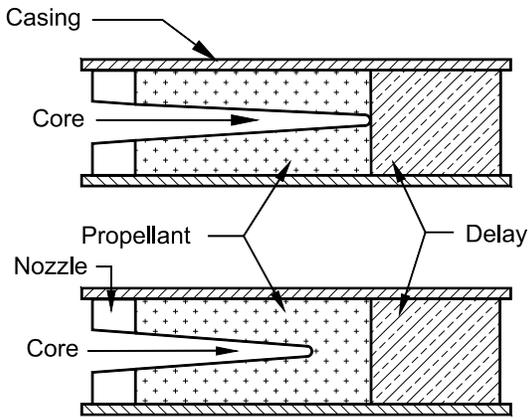
Figure 3. Rocket motors with varying core length.
