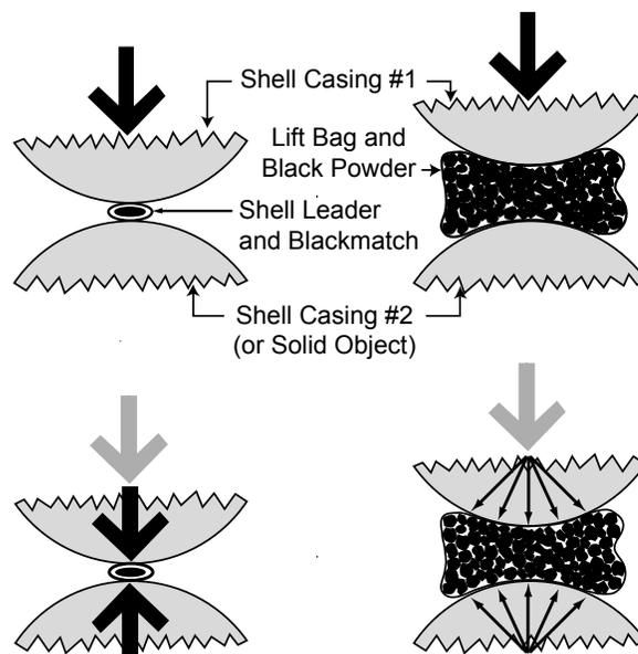
Figure 1. Sketches illustrating two possible impact scenarios occurring between two aerial shells: left, an impact with a shell leader at the point of contact; right, an impact with a bag of lift powder at the point of impact.
