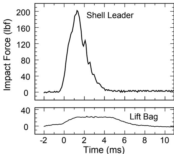
Figure 2. A graph of data demonstrating the substantial difference in the impact forces delivered to an electric match size object in collisions between two aerial shells with a shell leader and with a bag of lift powder at the point of contact.
