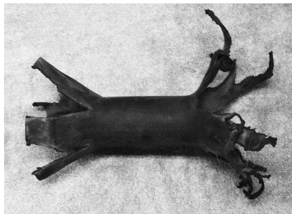
Figure 1. A photograph of a HDPE mortar following the explosion of a salute near its muzzle end (to the right).
