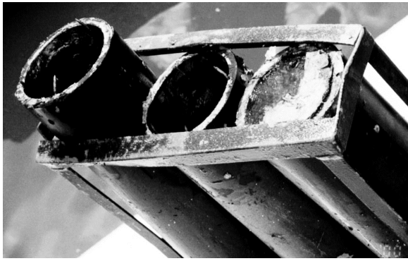
Figure 3. A photograph of the bottom of one of the mortar racks in which two of the three mortars had completely lost their plugs.
