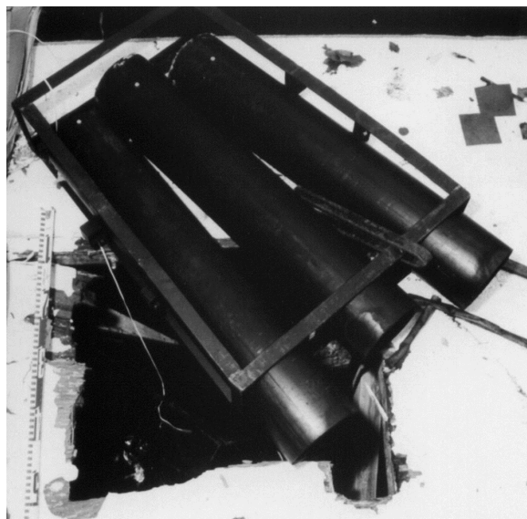
Figure 1. A photograph of deck of the wooden barge, with one of the three mortar racks partially covering the hole in the deck.
