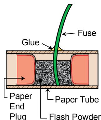
Figure 1. A photograph and cross sectional drawing of the test salutes used in this study.
