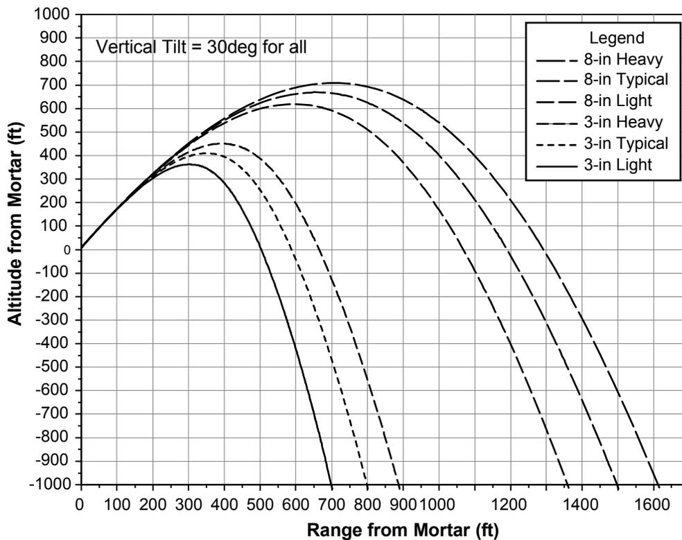
Figure 12. Comparison of trajectories for 76 and 205 mm (3 and 8") of three different masses (-20%, typical and +20%) (2500 ft above sea level, 50° C, 50% RH).
