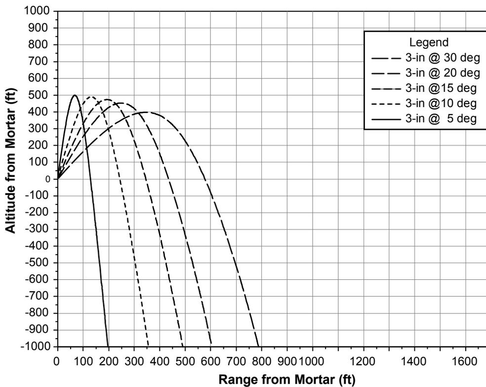
Figure 6. Trajectories for 76 mm (3") shell (2500 ft above sea level, 50° C, 50% RH).
