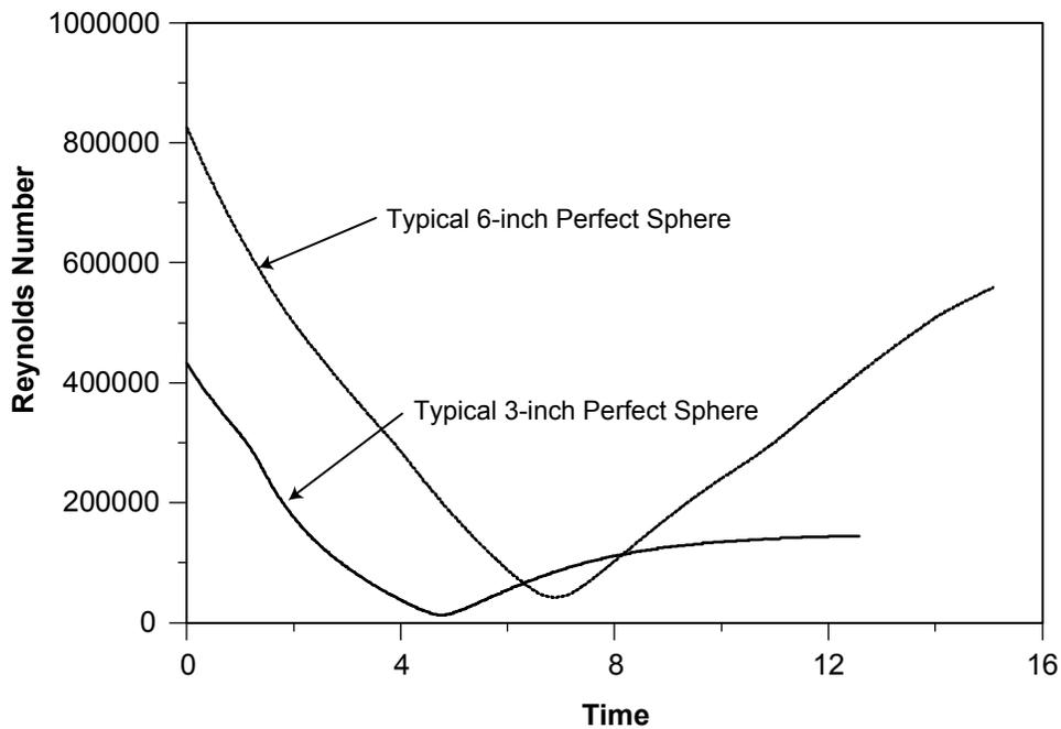
Figure 5. Perfect 76 mm (3") and 155 mm (6") spheres launched near vertical and with masses and velocities typical of aerial shells
