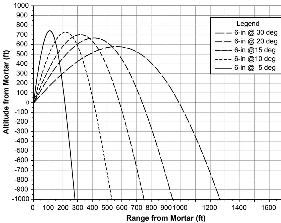
Figure 9. Trajectories for 155 mm (6") shell (2500 ft above sea level, 50° C, 50% RH).
