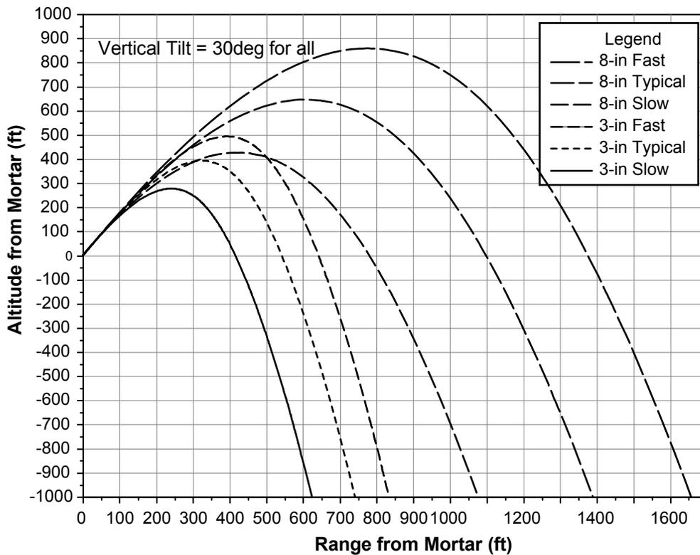
Figure 13. Comparison of trajectories for 76 and 205 mm (3 and 8") with launch velocities of 68, 91 and 113.6 m/s (225, 300 and 375 ft/s) (-20%, typical and +20%) (2500 ft above sea level, 550° C, 50% RH).
