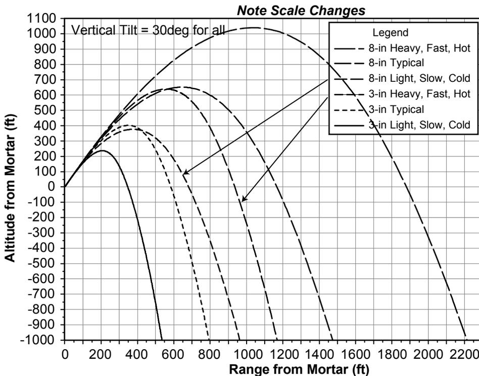
Figure 14. Comparison of trajectories for 76 and 205 mm (3 and 8") with extreme mass, velocity and altitude.
