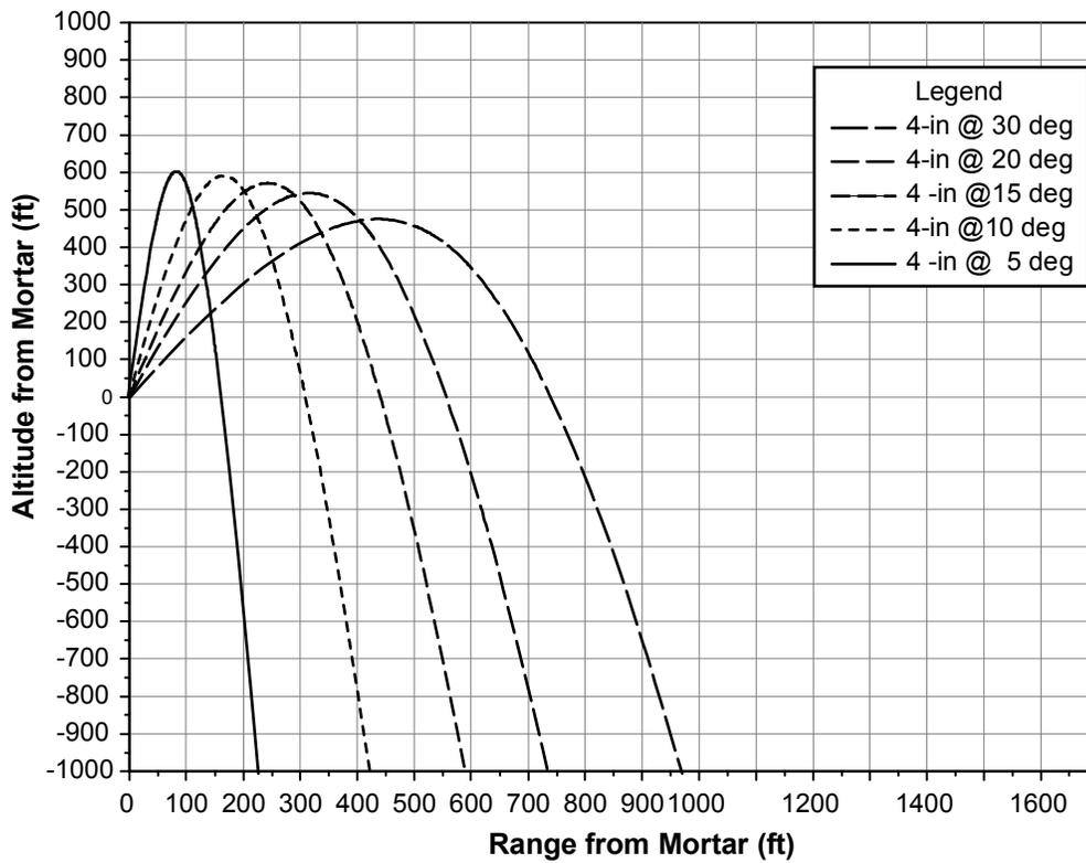
Figure 7. Trajectories for 101 mm (4") shell (2500 ft above sea level, 50° C, 50% RH).
