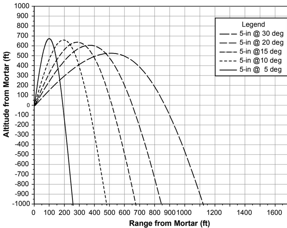
Figure 8. Trajectories for 127 mm (5") shell (2500 ft above sea level, 50° C, 50% RH).
