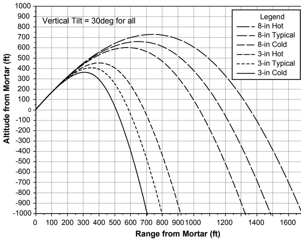
Figure 11. Comparison of trajectories for 76 and 205 mm (3 and 8") shells at extreme temperature and altitude.
