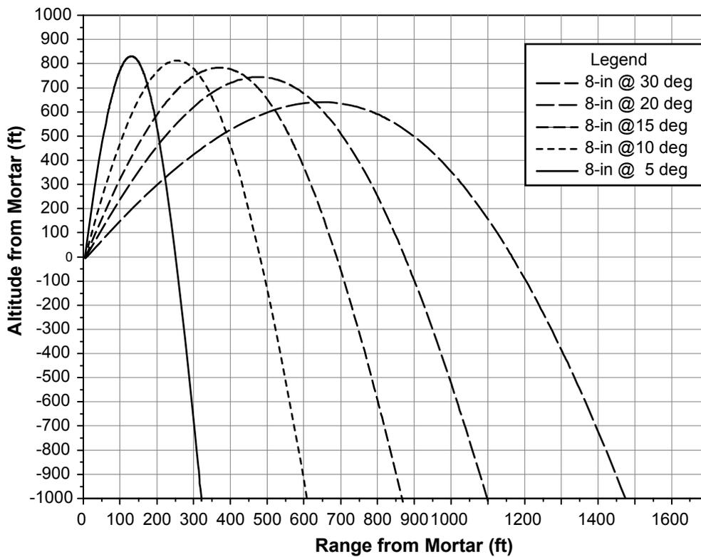
Figure 10. Trajectories for 205 mm (8") shell (2500 ft above sea level, 50° C, 50% RH).
