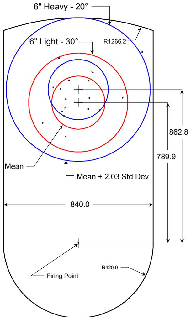
Figure 3. A plot showing the impact points for both low and high mass 155 mm (6") shells fired at off-vertical angles of  $20^\circ$  and  $30^\circ$ .
