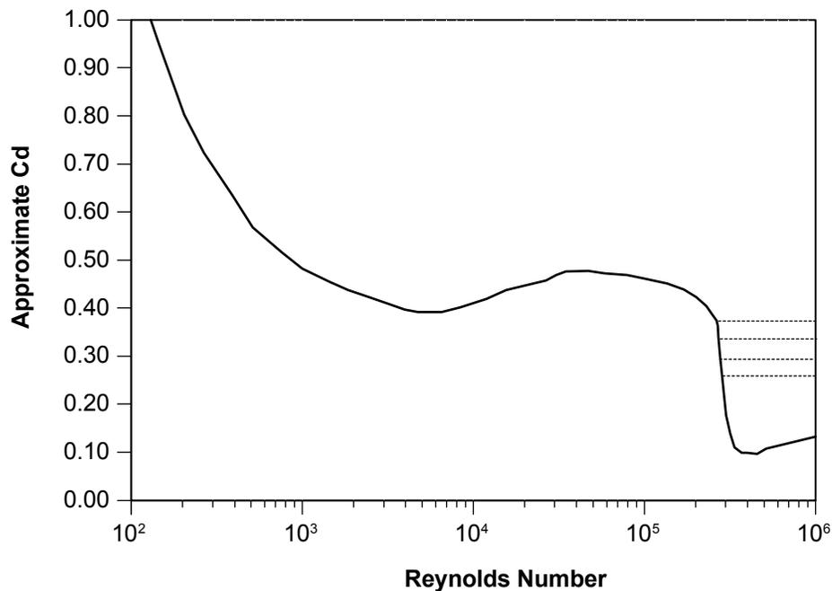
Figure 4. Approximate coefficient of Drag as a function of Reynolds Number.
